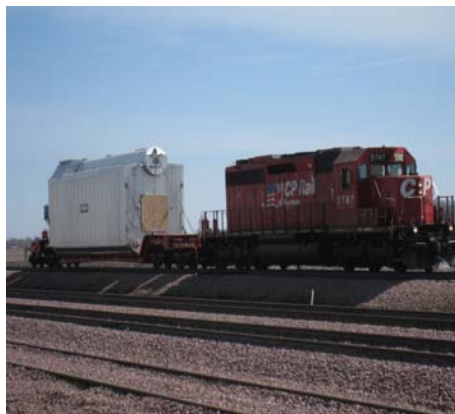
Delivering the Boiler via rail
